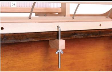
Clamp the back rail of the loom to a table. Insert the clamp into the centre hole on the back rail.
