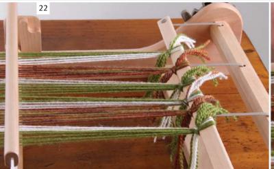
Tie the other groups in the same way. Check the tension. The tension of the threads should be the same. Tighten all the threads by winding the front handle towards you. Adjust the knots until all groups are the same tension.
