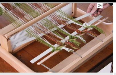
There are 2 weaving positions. First lift the reed into the up weaving position. Insert a cardboard warp stick into the shed. Slide it to the front of the loom. Change the reed to the down weaving position. Insert a cardboard warp stick into the shed. Slide it to the front of the loom.
