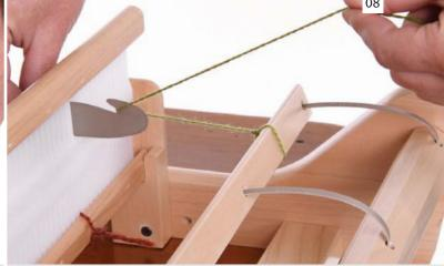
Push the threading hook through the same slot as the thread marker. Catch the yarn with the hook and pull a loop through the slot.
