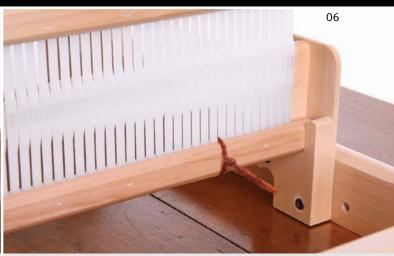
As a guide tie a coloured marker in a slot. 40cm (16ins) loom - 9 slots from one end. 60cm (24ins) loom - 24 slots from one end. 80cm (32ins) loom - 39 slots from one end.
