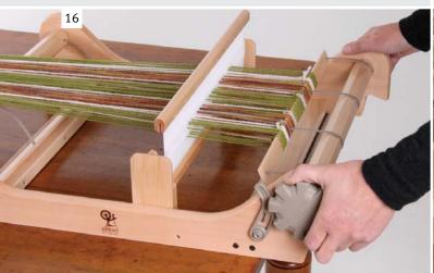
Stand at the back of the loom. Wind the back handle towards you until the back warp stick goes around the roller once.
