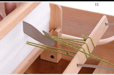
Go to the next slot. Take the yarn OVER the back stick, through the slot and over the warping peg. Continue this way, one yarn thread under, one thread over until you have 42 double loops/yarns through the slots (84 ends).
