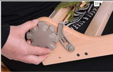
Keep the tension on the back handle and turn the front handle towards you until your work is approx. 5cm (2ins) from the roller. Click the **back** pawl down and retension the warp. As you weave continue winding your work onto the front roller in this way.
