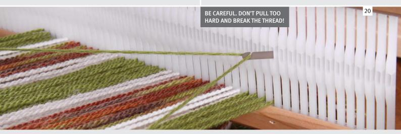
Lift the first 2 threads on the left to the top of the slot. Look behind the reed and gently pull the left hand thread out of the slot. The other thread stays in the slot.
