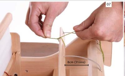
There are 84 warp ends in this scarf. That is 42 double threads that first go through the slots in the reed. Tie the warp yarn to the back warp stick directly behind the coloured thread marker. The back warp stick should be approximately 8cm (3½ins) from the back roller.
