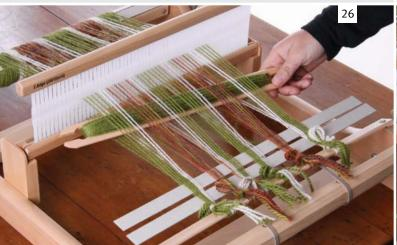
Change the reed to the up weaving position. Take the shuttle and pass it through the shed.
