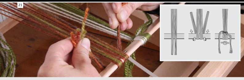
Turn the handle until the front warp stick is approx. 5cm (2ins) from the front roller. Divide the threads into 8 groups. Start with a centre group. Take the group of threads over and around the front warp stick. Divide it in two. Tie in a flat SINGLE knot.
