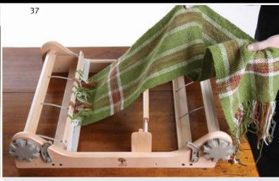
Release the front pawl and unwind the weaving from the front roller.
