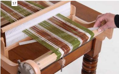
Insert a cardboard warp stick or piece of paper the full width of the loom.
