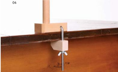
Clamp the warping peg to the other end of the table. Note: If the table top is not deep enough, place the end of the clamp over the warping block.
