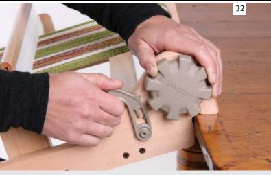
Continue weaving as per the last 2 rows until your work is approx. 8cm (3ins) from the reed. Now it is time to wind the weaving onto the front roller. PLACE THE REED INTO THE REST POSITION. Release the tension on the warp by turning the back handle away and click the pawl up.
