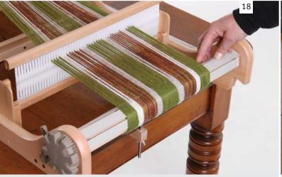
The cardboard warp sticks or paper separate the yarns and keeps the tension even. Add more cardboard warp sticks or paper as you wind the warp on.
