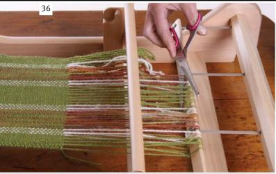
Cut the warp yarns along the back warp stick. Take care not to cut the warp stick ties. Cut the weft yarn and leave the end out.
