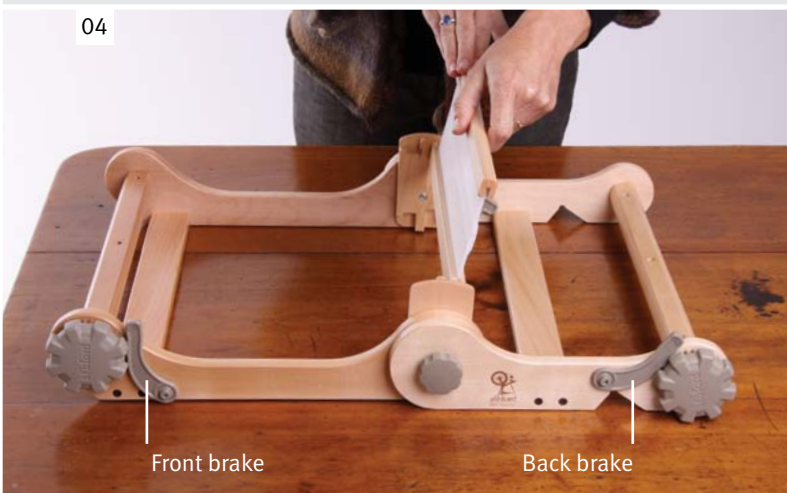
Place the reed into the rest position. Make sure the front and back brakes are on. When we say put the brake on, we mean the pawl should be clicked into the ratchet on the handle.
